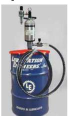
The new Viper Mk II kit includes an upgraded lubricant pump, built specifically for the Viper WRL. Two pump options are available the standard unit delivers 4.5kg/min. while the optional high volume unit delivers 13kg/min for fast lubrication of large diameter ropes, for further reduced down time.
